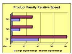
Large Signal = 70% of 1<sup>st</sup> Resonance Operation Small Signal = Frequencies extending past resonance, but at reduced modulation levels
